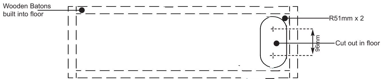
Fig. 17 Securing the Space Heater (Plan View)
