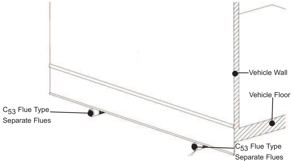
Fig. 41 Flue Type for Standard Installation C 53
