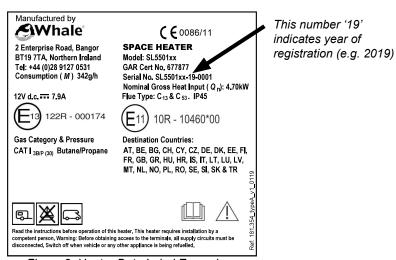
Figure 3. Heater Data Label Example
