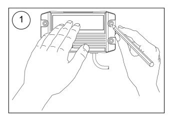
Mark the position of the four mounting spots. Remove the charger and drill the mounting holes. Fix the charger to the wall using corrosion resistant 4.8mm (3/16") dia. or M5 (#10) bolts, backed by a flat washer, and secured to the mounting surface with a split-ring lock washer.
