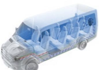
Evaporator vertical on the side at the rear
