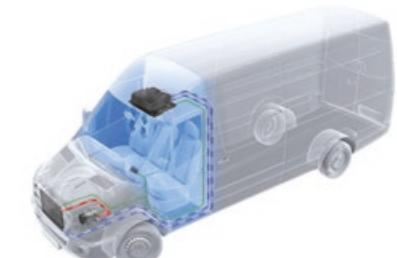
Evaporator integrated into the roof
