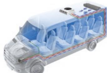
Evaporator under the roof
