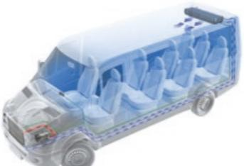
Evaporator under the roof
